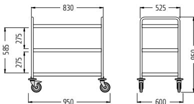
**Standard equipment:** Round-tube design, with 3 shelves made of stainless steel.
