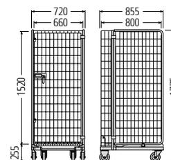
**Standard equipment:** Square tube frame chassis, welded. Hinged support surface made of wire mesh. Container structure of round-tube frame with wire mesh and plastic hinges. Door opening angle 270°.
