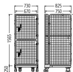
**Standard equipment:** Square tube frame chassis, curved. Hinged support surface made of square tube frame with wire mesh, reinforced with flat steel strips. Container structure of round-tube frame with wire mesh and plastic hinges. 2-part door with opening angle 270°.
