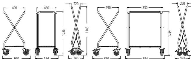
**Standard equipment:** Sturdy steel tube design with wire rack attached as support surface. Hook-and-loop fastener for polyester bag, flat steel retainer bar for plastic bag.
