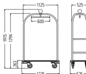
**Standard equipment:** Round-tube design with elegant 'crown' and coat rail. Sturdy platform with all-round bumper protection and deflectors, heavy duty, stain resistant carpet in anthracite.
