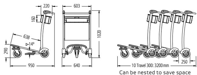
**Standard equipment:** Steel-tube design with sturdy luggage loading area. Self-adjusting, zero-maintenance brake. All-round bumper rail on the loading area. Practical basket for hand luggage or travel paraphernalia. Can be nested to save space.
