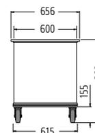
**Standard equipment:** Robust trolley made of anodised aluminium. The base shelf is raised and lowered automatically depending on the weight of the transported goods. This enables staff to load and unload the trolley comfortably and without straining their backs.
