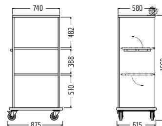
**Standard equipment:** Sturdy construction made of anodised aluminium. All-round plastic bumper. Roll-down front panel made of plastic as standard. Two 90° hinged shelves.
