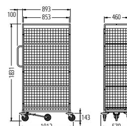
**Standard equipment:** Chassis made from square tubing. Side panels made up of square tubing frame with wire rack inserted into chassis and screwed into place. 4 adjustable shelves. 4 large deflectors to protect the furniture.
