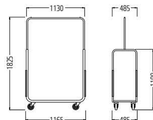
**Standard equipment:** Round-tube design with robust loading area for luggage. Plastic profiles mounted at the side on the upright struts to protect the interior décor.
