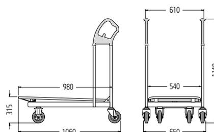
**Standard equipment:** Frame made of flat oval tubing, round-tube bars with ergonomically shaped handles made of shatterproof plastic. Frost- and water-resistant wooden platform with all-round protective frame made of square tube.
