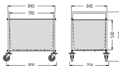
**Standard equipment:** Steel-tube design with sturdy wire rack as support surface. Practical all-round hook-and-loop fastener for securing the large polyester bag, optionally with cover.
