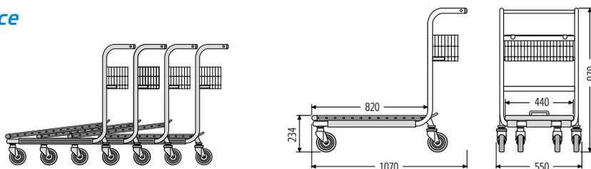
**Standard equipment:** Can be nested to save space. Frame made of flat oval tubing. Wire platform with double edging wire. With close-meshed wire basket.
