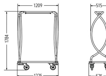
**Standard equipment:** Round-tube design with coat rail. Sturdy platform with all round bumper and deflectors, heavy-duty, stain resistant grey melange carpet.
